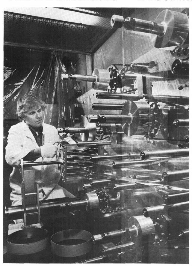
THIS COMPLEX MACHINE winds mylar and aluminum foil into energy storage capacitors for firesets. Ron Cheek (2153) trims aluminum foil before attaching it to circular frame like one shown at lower right. Capacitors like one at lower left are automatically wound. Firesets are one major area of design and development in Microelectronics Directorate 2100.
